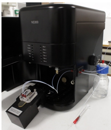
Figure 7-1: Loading a sample with the LVFC.
