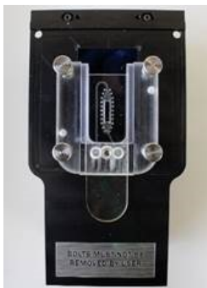
Figure 5-8: Low Volume Flow Cell assembly mounted on laser module with sprung fastening bolts.
