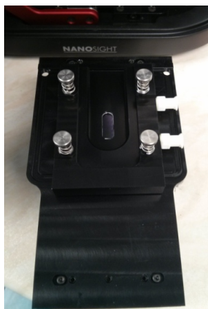
Figure 12-8: Laser module with O-Ring TopPlate unmounted from the NS300.
