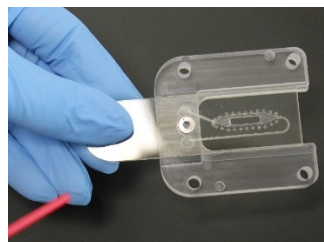
B: Drying the chamber seal on the underside of the gasket component
