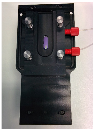
Figure 5-13: O-Ring top-plate with tubing fittings for syringe pump use.
