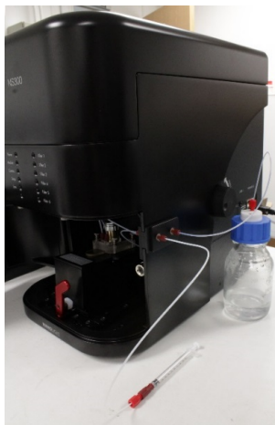
Figure 5-15: External NS300 fluidic connections.
